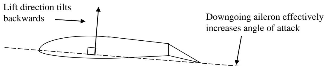
In the case shown, the downgoing aileron (on the outside of the turn) effectively increases the angle of attack of the outer wing, tilting the lift vector backwards as shown. An upgoing aileron obviously has the opposite effect, reducing the effective angle of attack and tilting the direction of the lift force forwards. In addition to the change in direction of the lift forces, both ailerons also increase the drag on the model when they move since they are effectively small airbrakes.
